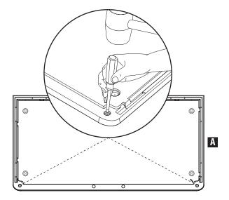
Drill pilot hole through top surface of floor, 2 places on Front Floor (A).
